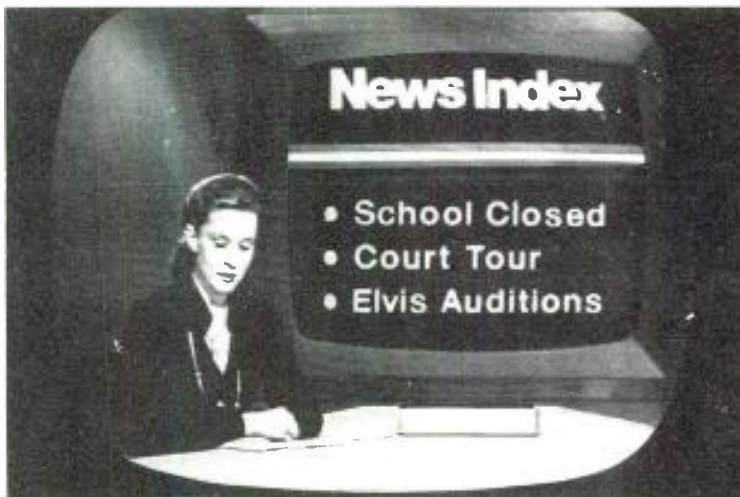
The above title card was created by a graphic artist with news items added by the Chyron II, and stored as a composite on the ESP. Display of the composite is routed through the DVP to take advantage of auto chroma key tracking
